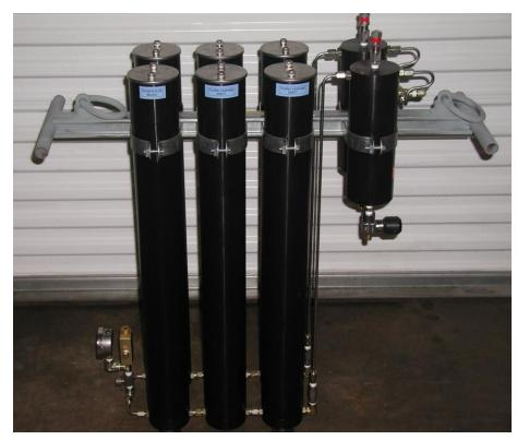
This system should be considered the minimum size for a 50 CFM compressor
